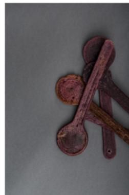
The waste is dried and then blended into a paste before being 3D-printed
