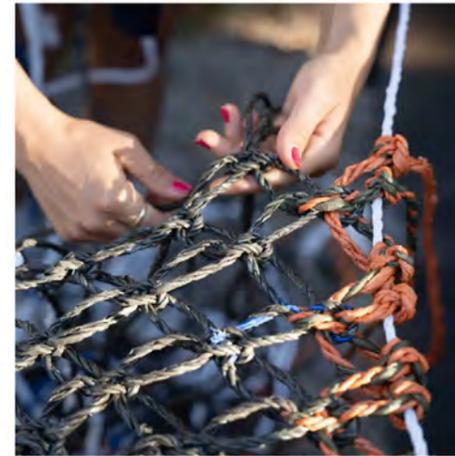
The rope is knotted together into a net using a macramé technique
